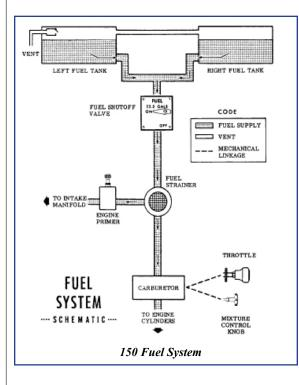
the fuel selector. It is certainly very disconcerting to be flying along and watch your left fuel gauge going down while the right fuel gauge continues to indicate full. The funny thing about this situation is that while only the left gauge is showing fuel usage, the engine may very well be using fuel from the right tank!
