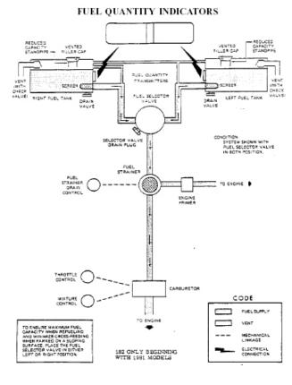
182 with integral tanks, dual wing vents and right fuel feeds line vented to right tank 1981 and up.
